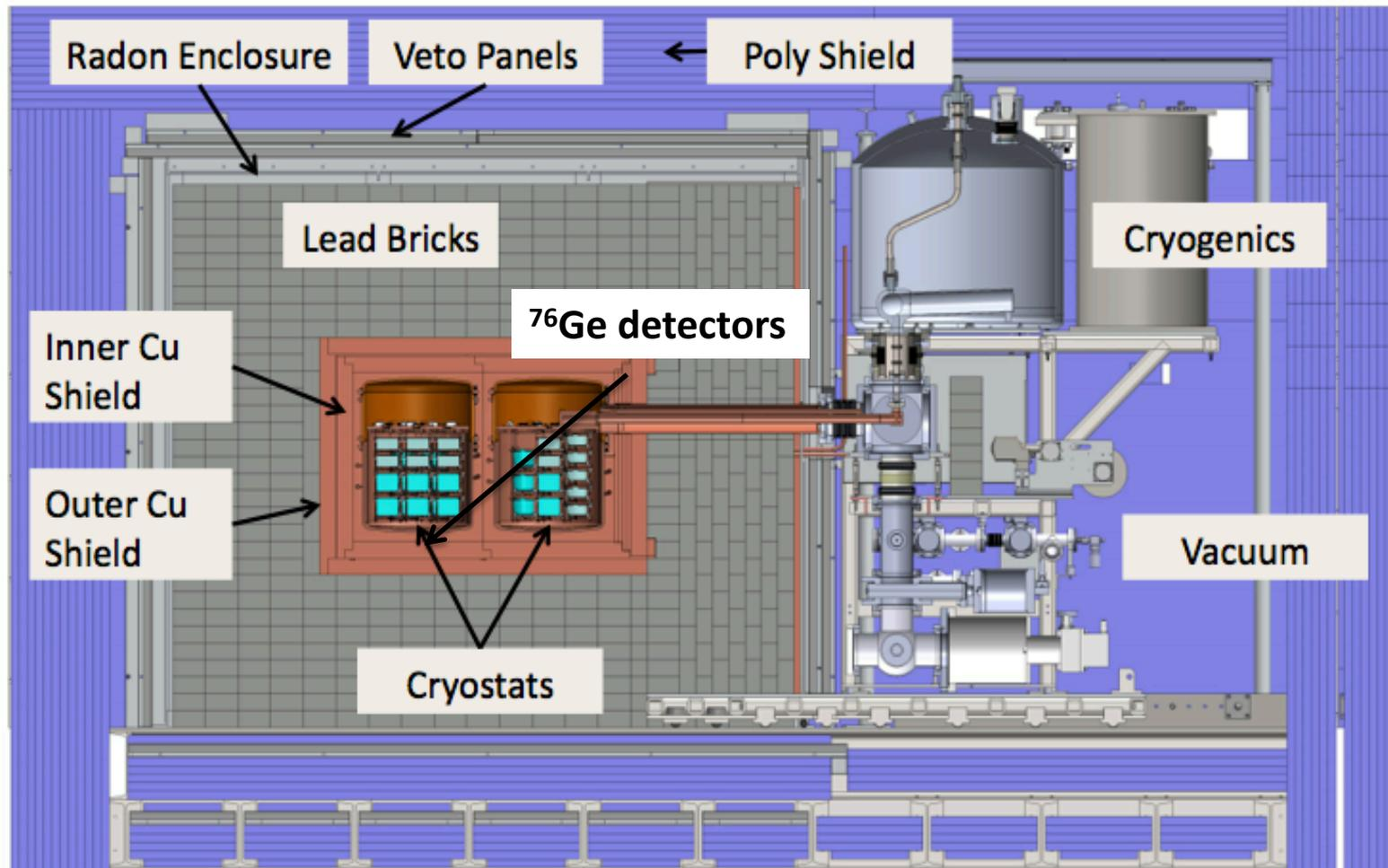
~ 30 kg of Isotopically Enriched  $^{76}\text{Ge}$  detectors located at ultra quiet conditions with minimum radioactive background.
