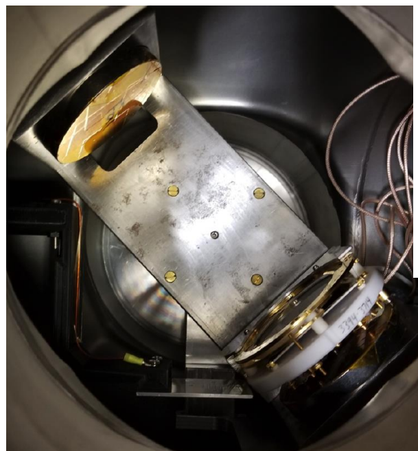
MCP tracking detector used for ^{84}\text{Se}(d,p) experiment
